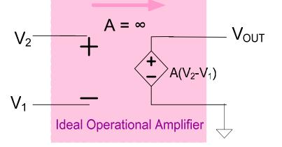
"E" source model in SPICE or SPECTRE can be used to model the Op Amp
