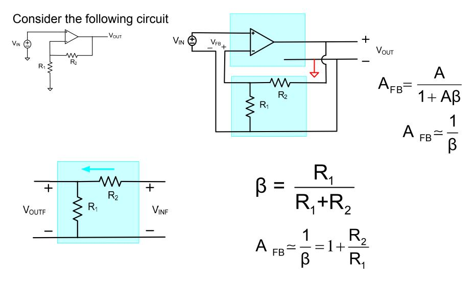
Observe this serves as a basic finite-gain noninverting amplifier
