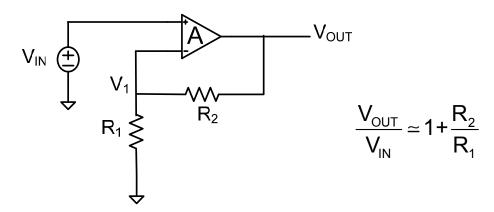
If  $R_2/R_1 = 9$ , how much error was introduced by assuming A= $\infty$  if the actual op amp has a gain of A=10<sup>5</sup>?
