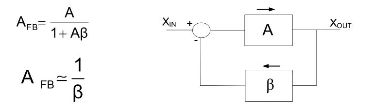
Feedback has shifted the performance requirements from the A amplifier to the  $\beta$  amplifier.
