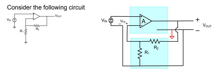
For  $R_{IN} = \infty$  and  $R_0 = 0$ , this is an EXACT representation of Black feedback structure
