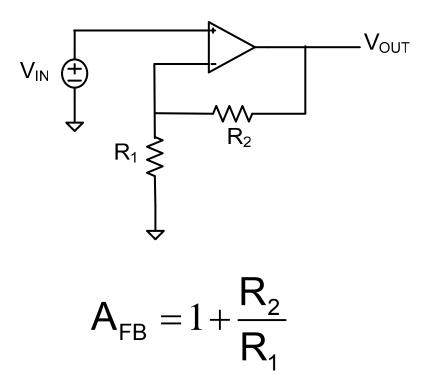
Gain can be accurately determined by resistors
